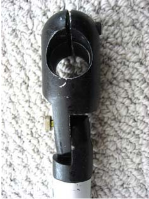
Split head for sensor adjustment; pivot pull pin for 5 point head adjustment
